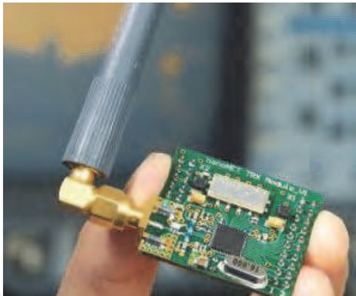
Fig. 5. An active RFID tag with a changeable antenna
