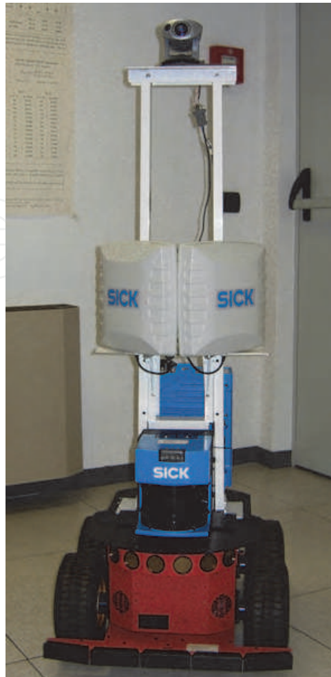
Fig. 1. The mobile robot Pioneer P3AT equipped with two RFID antennas and a laser range scanner.
