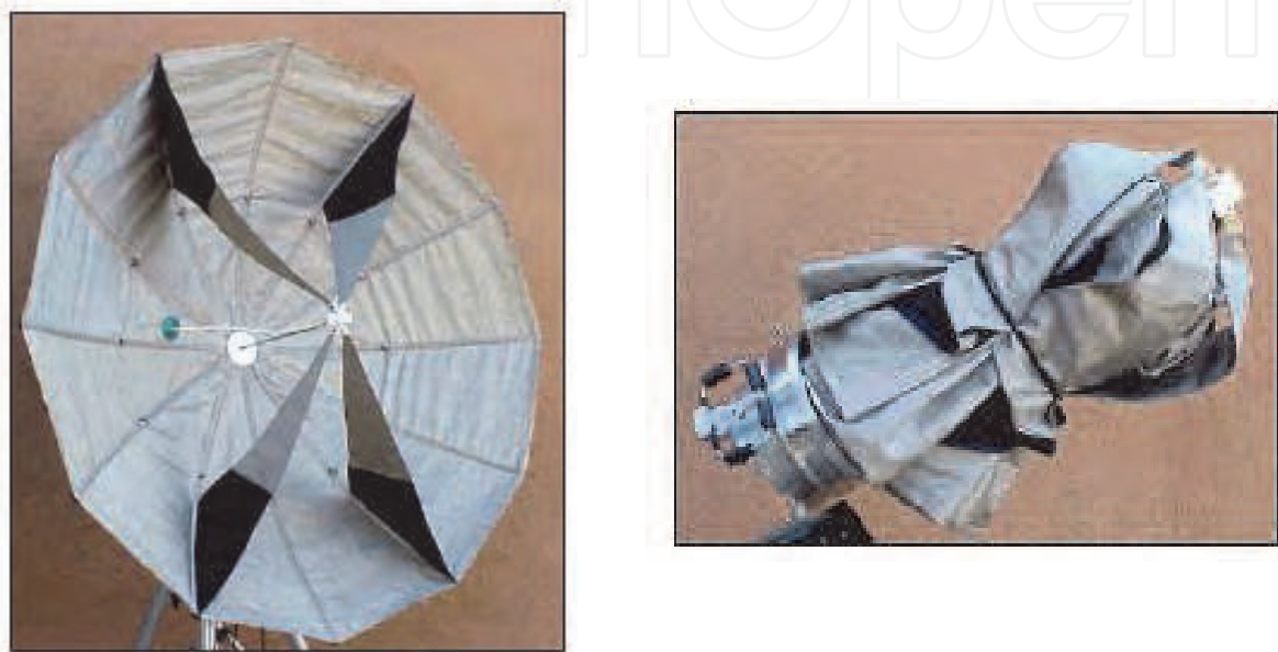
Fig. 2. U-CIRA1 antenna developed by Farr Research (USA)
