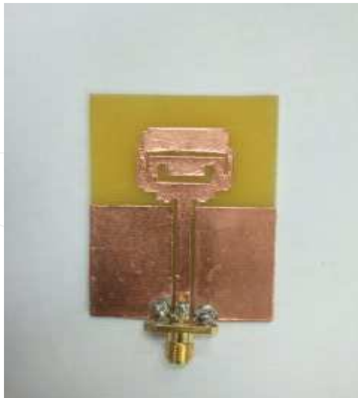
Fig. 2. Photograph of the implemented antenna.
