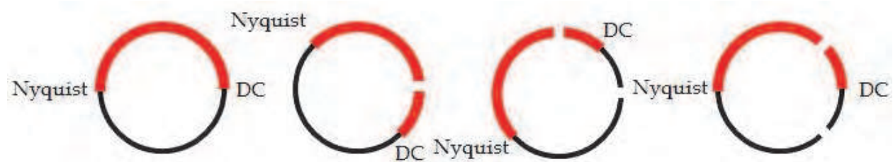
Fig. 10a. Input X(z) Fig. 10b. Rotate \omega_0 to DC Fig. 10c. Rotate -\omega_0 to DC Fig. 10d. Rotate back
