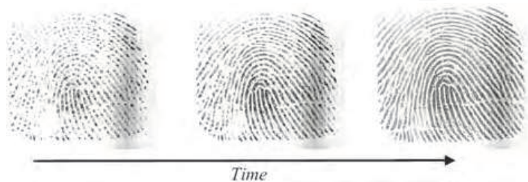
Fig. 2. Example of live fingerprint images acquired some time apart (Schuckers et al., 2003).
