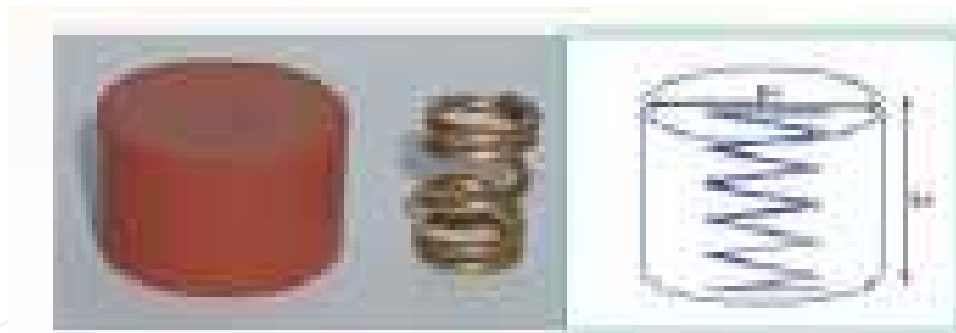
Fig. 17. Example of Composite Rubber/SMA spring damper
