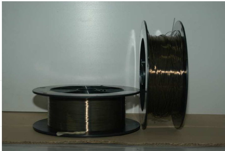
Fig. 3. The photograph of the super elastic SMA wire samples (Available in spool form)
