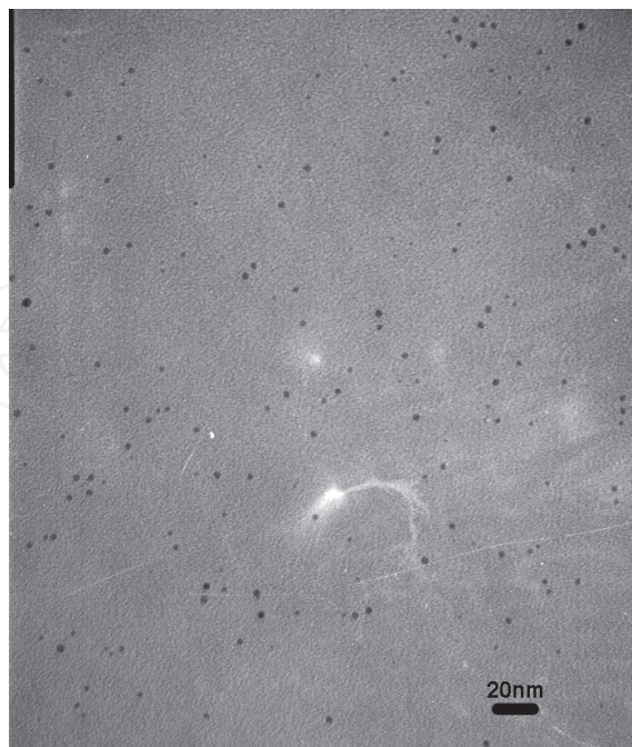
Fig. 7. The scheme of the formation of lysozyme-stabilized gold nanoparticle (up) and the TEM image of the as-formed gold particles (bottom).
