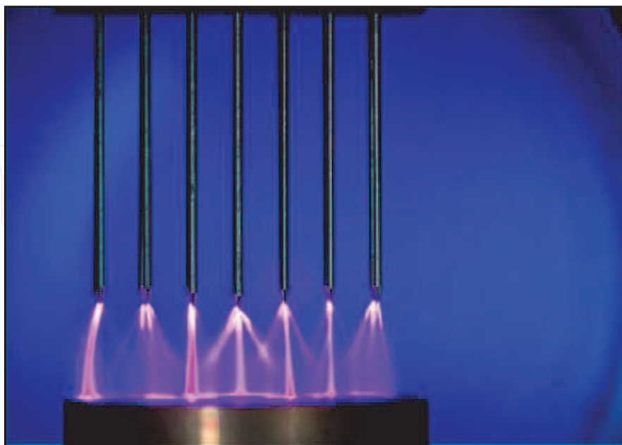
Fig. 3. b. View on a multi-tip pulsed corona discharge tested at LAPLACE-PRHE Laboratory.
