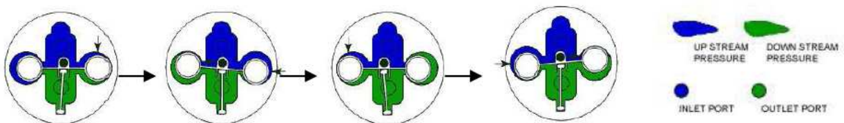
Fig. 8. Flow measurement principle for the flow meter. Pistons movement inside the chamber while the liquid passes through the flow meter (DEA, 2008)
