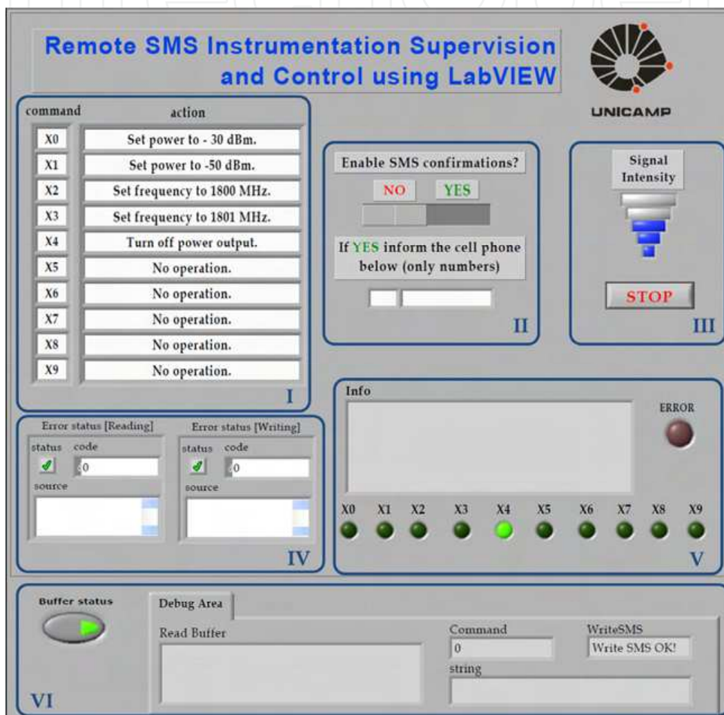
Fig. 18. The application GUI created in the LabVIEW front panel.
