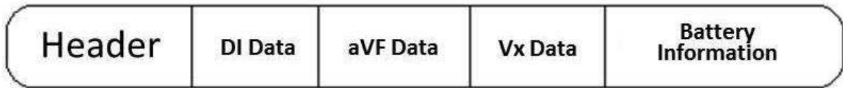
Fig. 11. Format of the data packet sent by the receiver to the RS-232 interface
