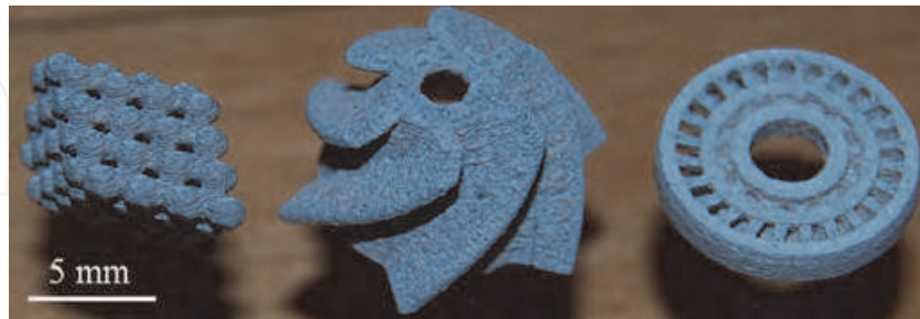
Fig. 17. Miniature ceramic parts by LSD-based direct laser sintering process, photonic crystal, blade wheel, and stationary blade
