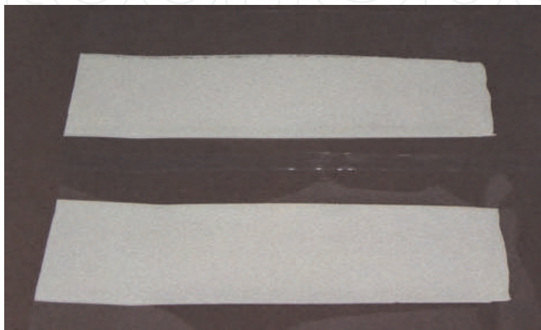
Fig. 12. Green tapes obtained by tape casting from the aqueous AlN-based suspensions.
