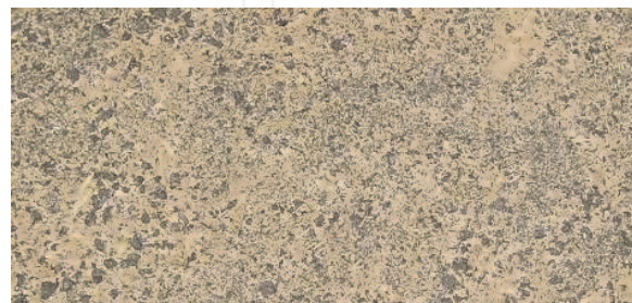
d) 15 % by mass sawdust with 85 % lignite mixture
