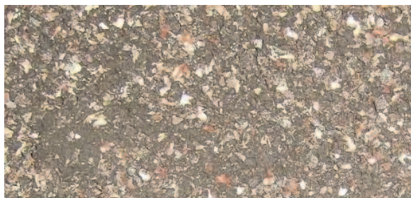
c) 15 % by mass corncob with 85 % lignite mixture
