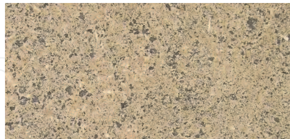
h) 30 % by mass sawdust with 70 % lignite mixture
