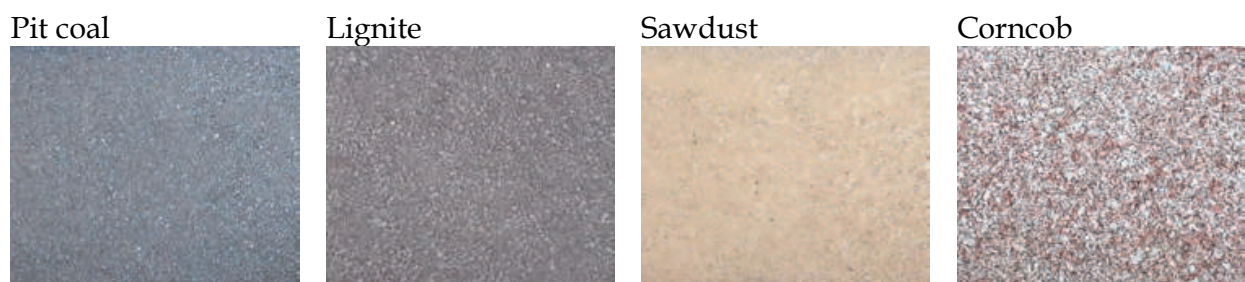
Fig. 3. Types of coal and biomass used as fuels for co-firing facility
