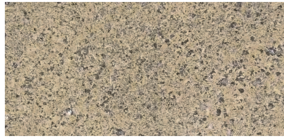
f) 30 % by mass sawdust with 70 % pit coal mixture
