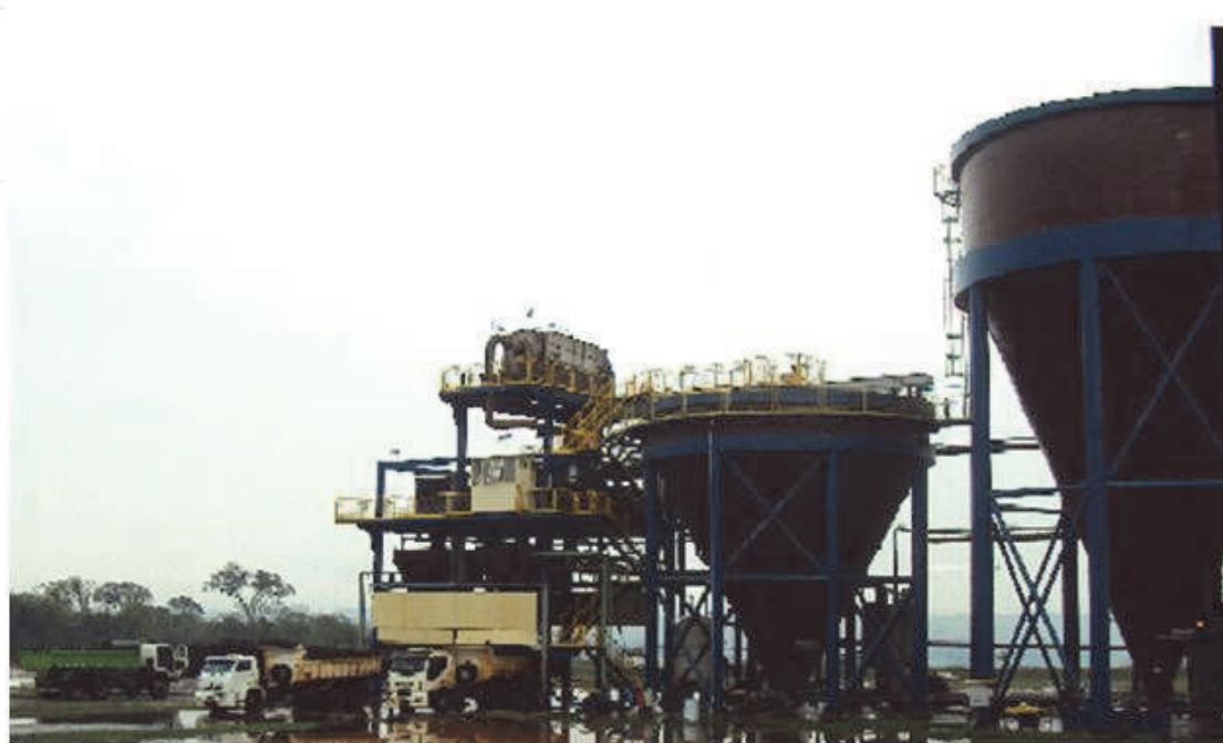
Fig. 4. System for treatment of water from gas washer to remove the ash using decanters and porous blankets.
