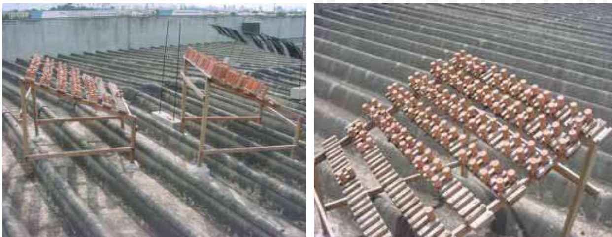
Fig. 11. Samples on terrace exposed on the roof directed to the best insulation direction according to the local coordinates
