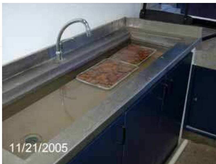
Fig. 10. Laboratory tank for wetting and drying cycling test
