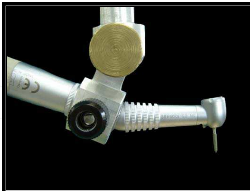
Fig. 4. The jig used to fix the handpiece to the vertical arm of the apparatus
