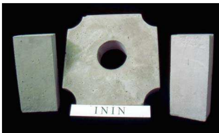
Fig. 9. Bricks and lattices obtained from granular solid residuals coming from diatomaceous, mining industrial residuals and binders
