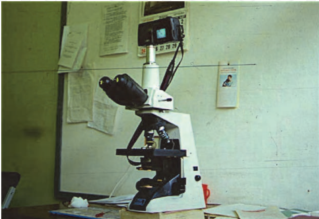
Fig. 10. The basic instrumentation for static telepathology is simple and inexpensive: a tricolour microscope coupled with a digital camera and a web connection.
