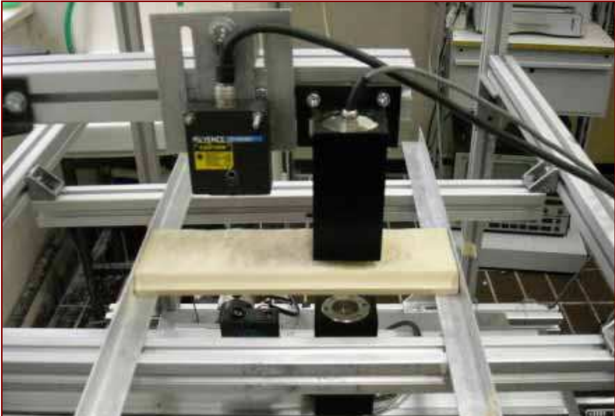
Fig. 14. The scanning system with ultrasonic and laser triangulation transducers
