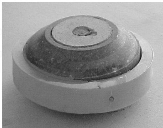
Fig. 3. Gasket with the PVC ring
