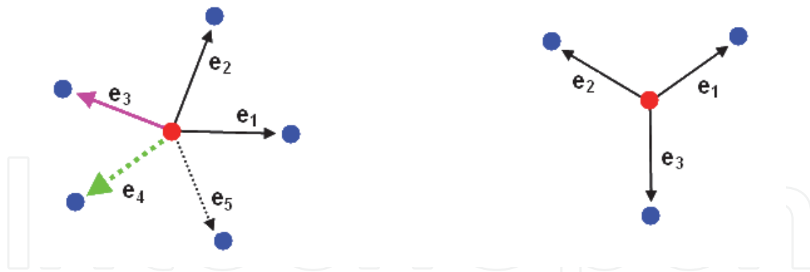
Fig. 14. On left the 5 first nearest neighbors in the pristine 4D hyperdiamond with the properties \|e_i\| = 1 and e_1 + e_2 + e_3 + e_4 + e_5 = 0 . On right, the 3 first nearest in pristine 2D graphene with \|e_i\| = 1 and e_1 + e_2 + e_3 = 0 .
