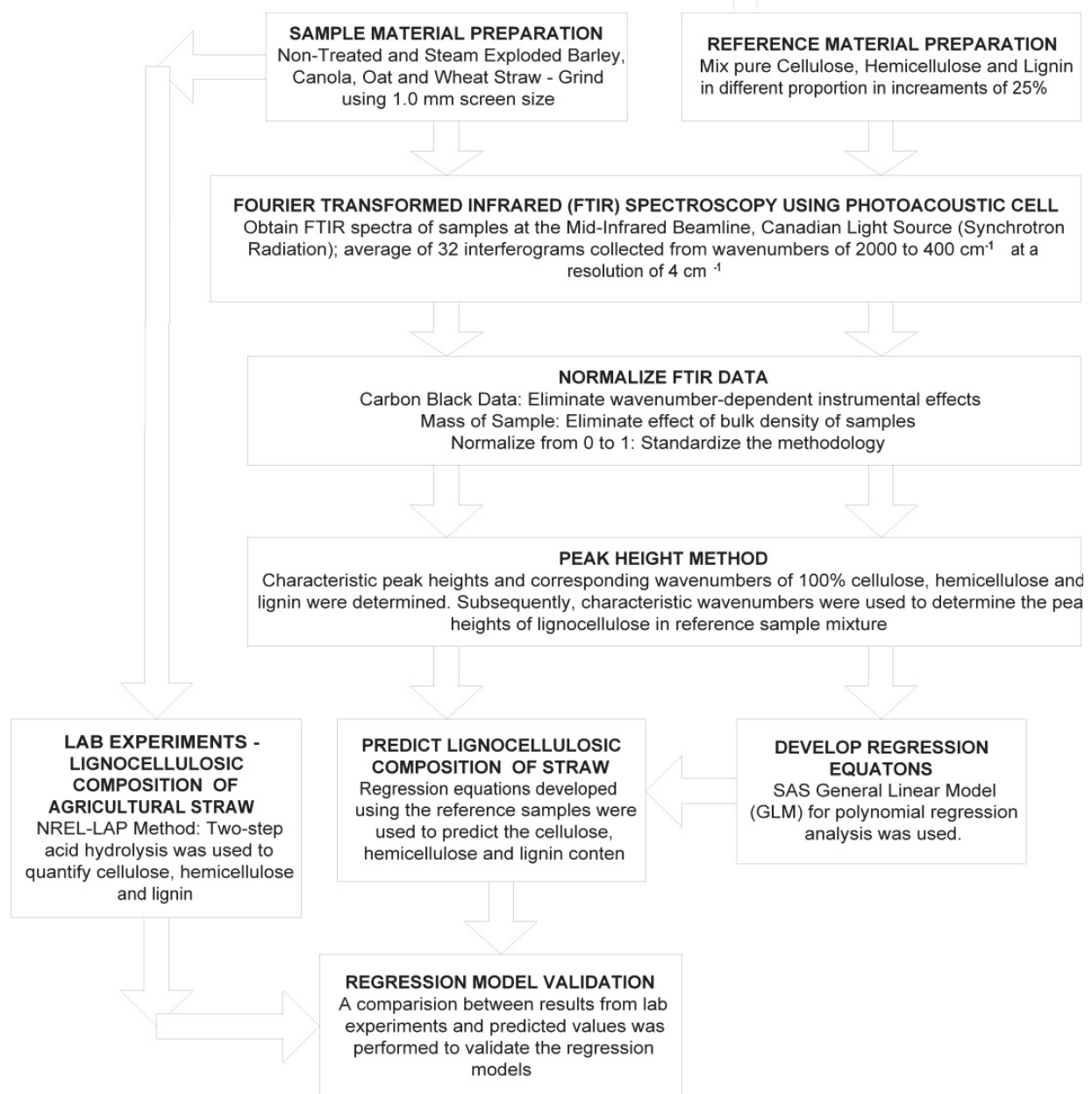
Fig. 3. Experimental procedure followed to characterize lignocellulosic composition of agricultural straw (Adapa et al., 2011b).
