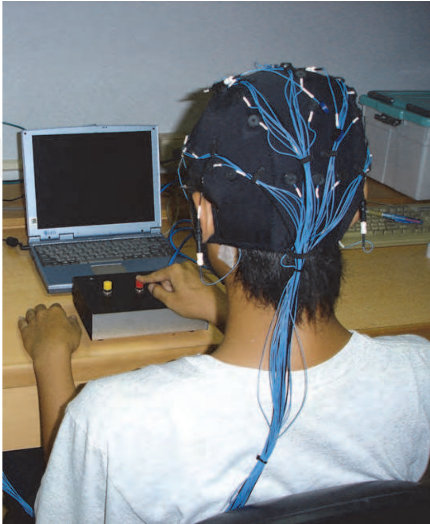
Fig. 3.3. A participant wearing an EEG cap with scalp electrodes performed the modified flanker task
