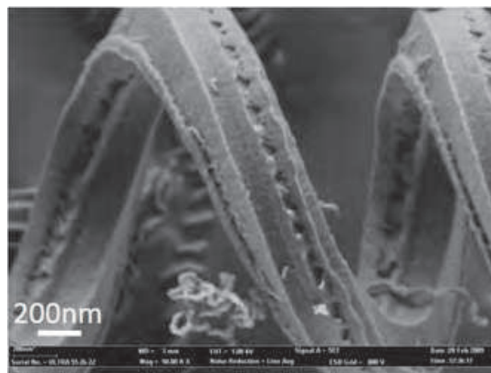
Fig. 21. SEM micrograph of CNC by the FE-SEM with a low acceleration voltage. Courtesy of Dr. Hamanaka at JFCC.
