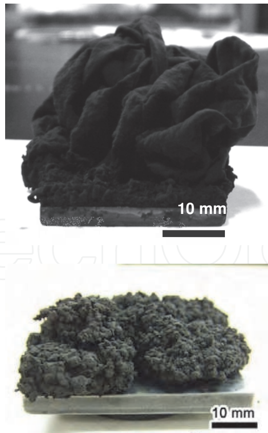
Fig. 19. Images of as-grown HCNFs synthesized by CVD. (a) CNCs using the Fe/Sn catalyst and (b) CNTws using the Fe/Sn catalyst.
