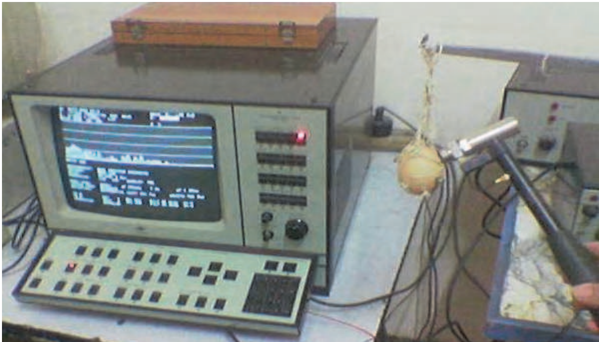
Fig. 3. (b) Free suspension for modal analysis.
