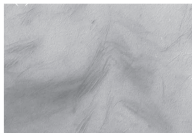
Fig. 5. Dispersion of modified nanoclay into poly \epsilon -caprolactone (PCL), from Labidi et al. (2010). Width of the picture is 250 nm
