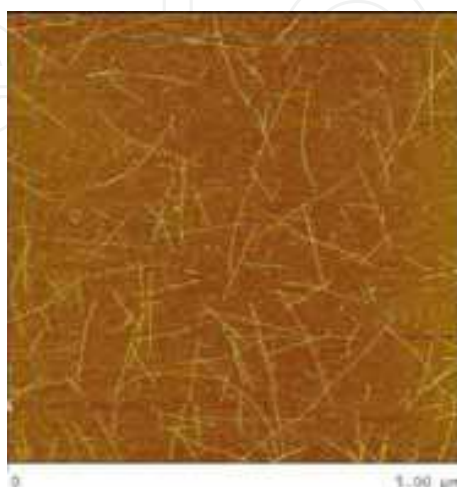
Fig. 7. Atomic force microscope image of synthesized imogolite.
