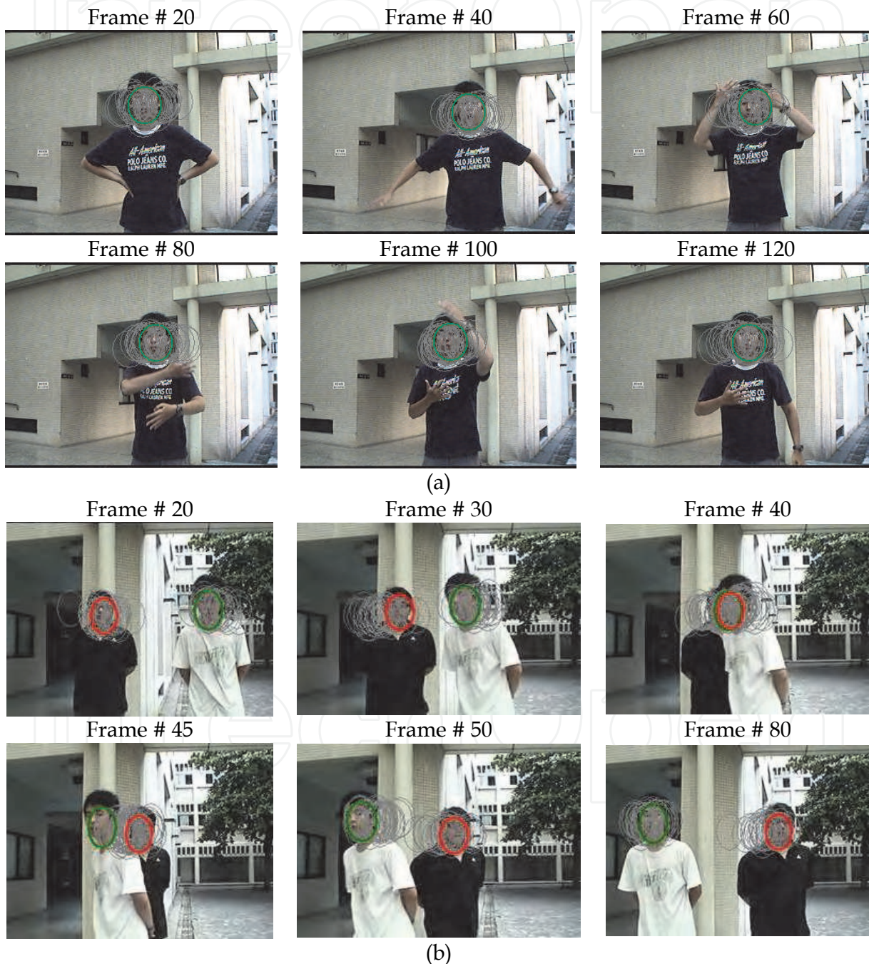
Fig. 9. Some face tracking results from using our real-time face tracking system for: (a) a single human; (b) multiple humans within the field of view of the PTZ camera equipped on the robot.
