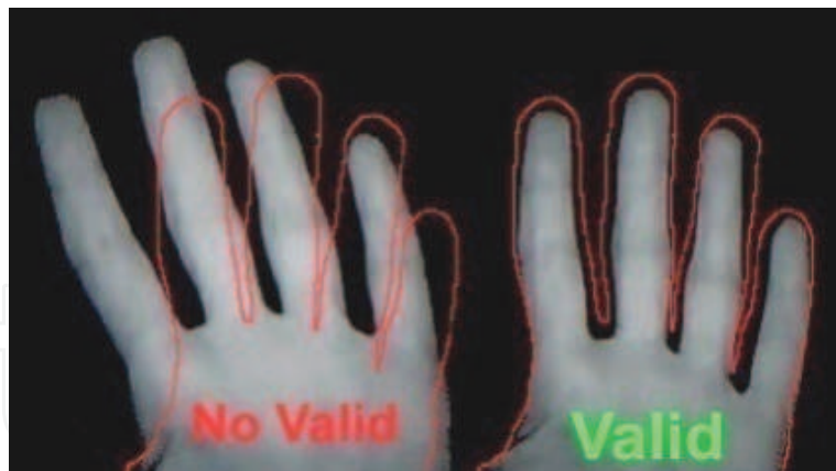
Fig. 3. Hand mask and hand overlapping. Valid stands for overlapping greater than 70%.
