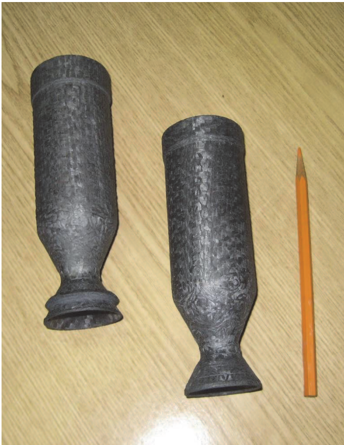
Fig. 7. Work material of ceramic combustion chamber.
