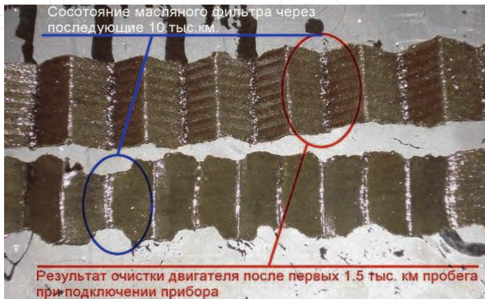
Fig. 16. Condition of the oil filters with the utilization of the ERF (above) and without it (below)
