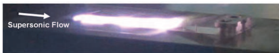
Fig. 3. Arc discharge picture in the supersonic flow.
