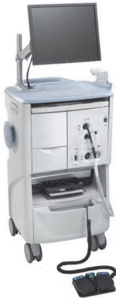
Fig. 4. Retcam instrument (Clarity Medical Systems) for retinopathy of prematurity screening
