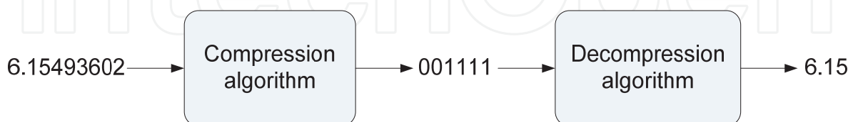
Fig. 3. Example of lossy data compression (Pu, 2006).
