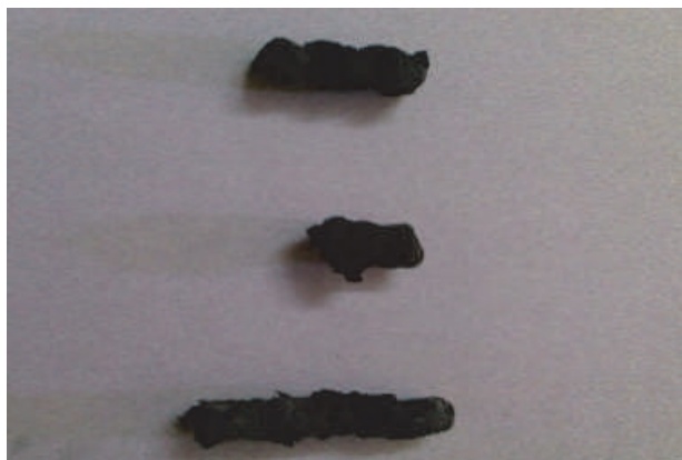
Fig. 2. Cigar like structure deposited on the Copper cathode during Arc evaporation process
