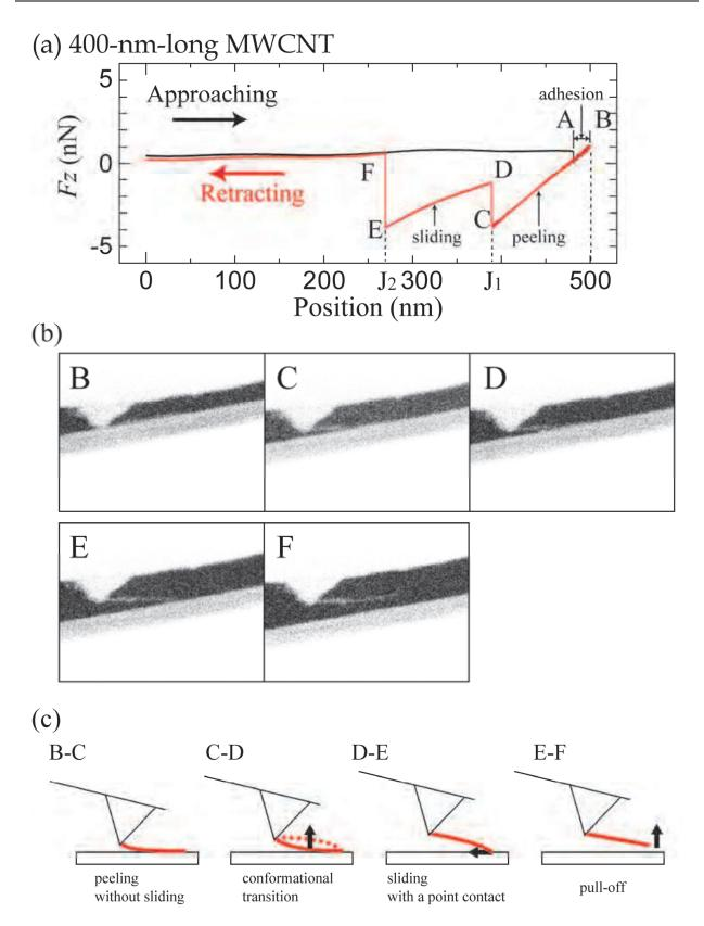
Fig. 2. (a) Vertical force-distance curve measured for the probe of a 400-nm-long MWCNT. (b) Several frames in the movie recorded during adhesion and peeling. (c) Schematic of (b).
