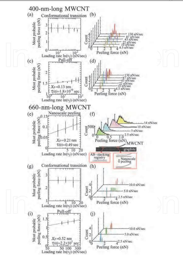
Fig. 5. The histogram of the peeling force, and the most probable peeling force f \* at various force loading rate,  $v_f$  for all the processes of the nanoscale peeling, conformational transition, and pull-off for 400-nm-long MWCNT and 660-nm-long MWCNT.
