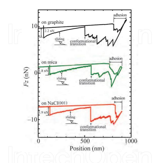
Fig. 6. Vertical force-distance curves measured on graphite, mica and NaCl(001) surfaces.
