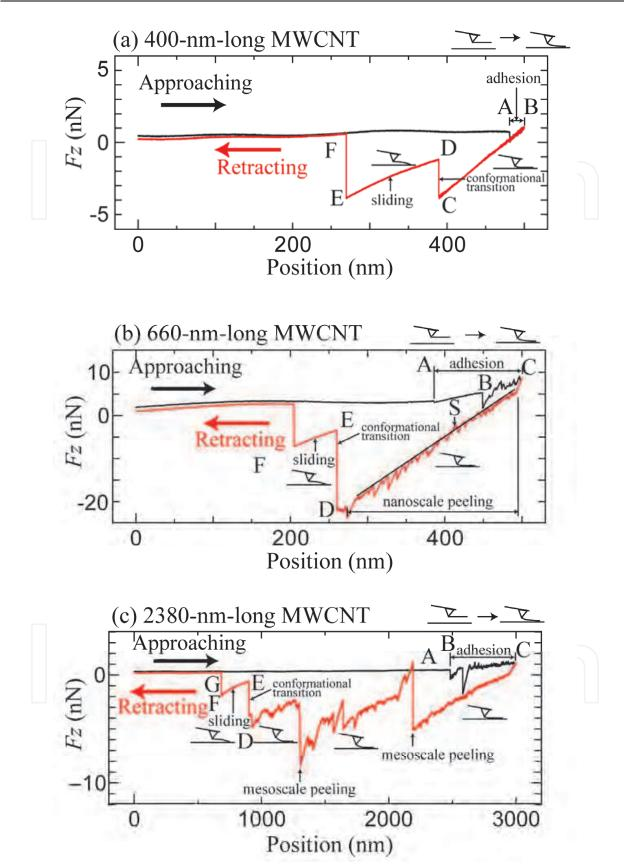
Fig. 3. Vertical force-distance curves measured using (a) 400-nm-long, (b) 660-nm-long, and (c) 2380-nm-long MWCNTs.
