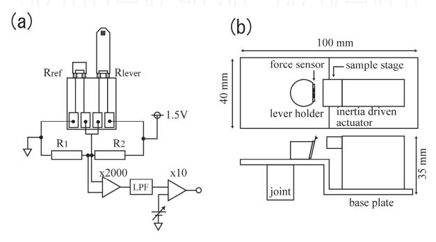
Fig. 1. (a) Schematics of a force detection system with self-detecting cantilever. (b) Overview of the force detection system. Force sensor and inertial driven actuator are fixed on the base plate. The signal from the sensor and the control signal of sample stage are handled by a computer via A/D, D/A compatible board. Thus, the signal is related to the motion of sample stage. SEM images can be recorded by using a video recorder as a movie.
