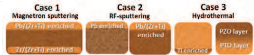
Fig. 7. Common compositional profiles for PZT thin film fabricated by sputtering and hydrothermal techniques. Case 1: based on the work of Vidyarthi et al., 2007; Case 2: Chang and He, 2005; Suchaneck et al., 2002; Case 3: Morita et al., 1997; Ohba et al., 1994.
