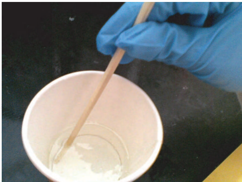
Fig. 3. Mixing of epoxy resin and hardener
