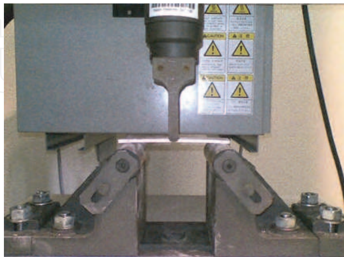
Fig. 10. Three point bending test setup
