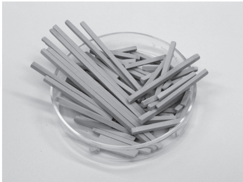
Fig. 9. General view of granulated \text{Al}_2\text{O}_3/\text{Al} composites prepared from powdered TCA and PA-4 used as supports for dehydrogenation catalysts.
