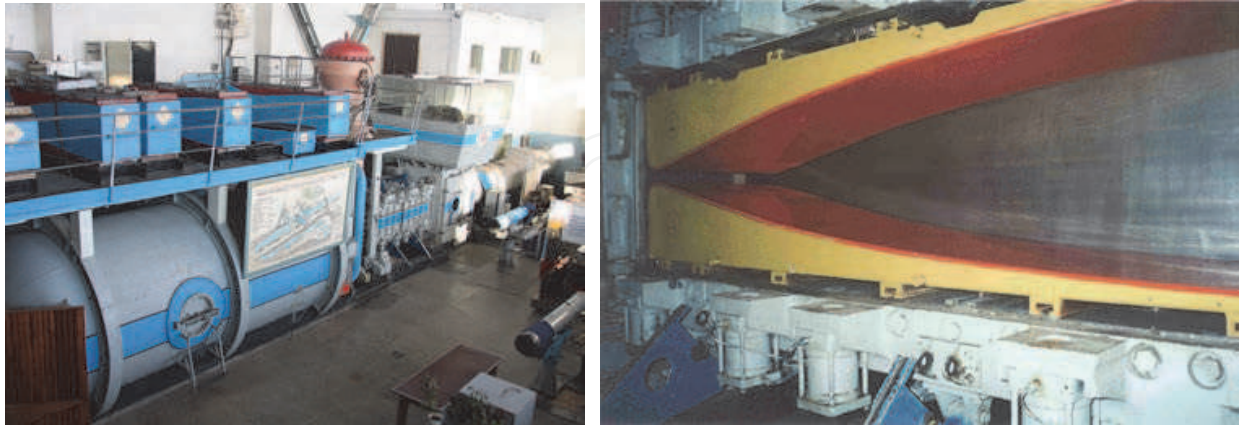
Fig. 1. T-313 supersonic wind tunnel and the nozzle unit with changeable profiled inserts for the Mach number M = 4.0 .
