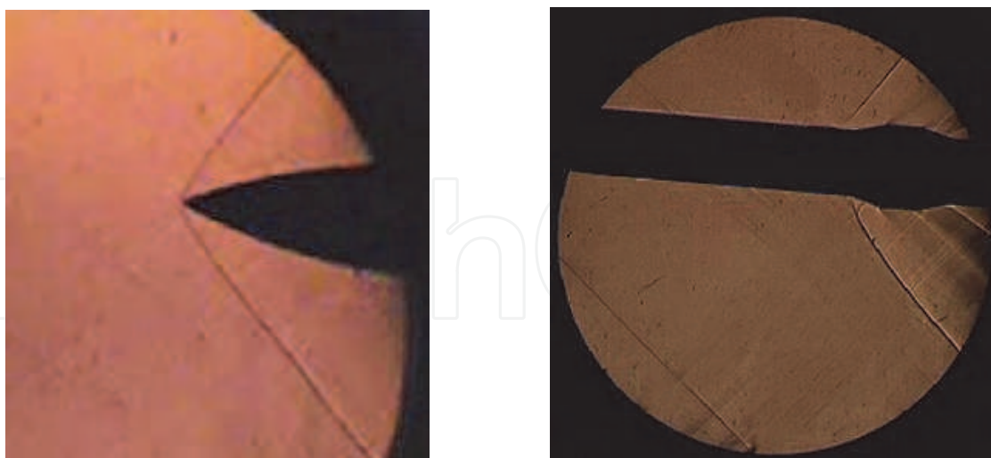
a) Oblique shock in the nose region of the model b) Compression and expansion waves around the large belt ( 15^\circ )
