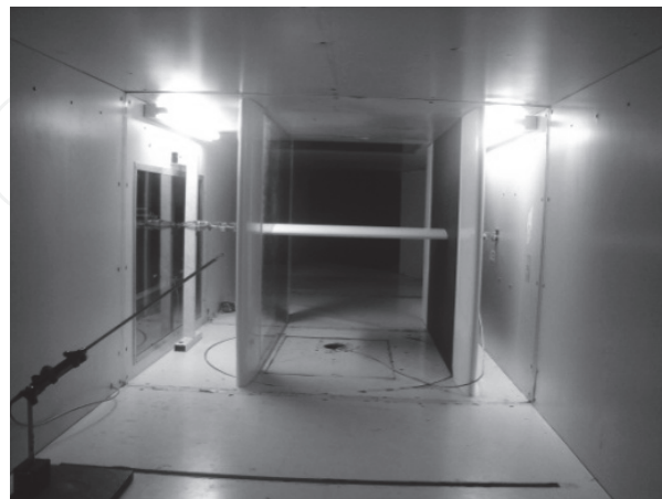
Fig. 3. Test section and Measuring equipment
