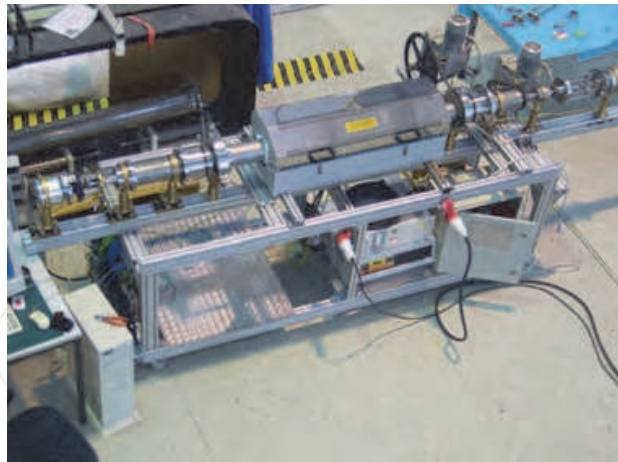
Fig. 25. Photograph of the high temperature rotary kiln reactor for char activation.
