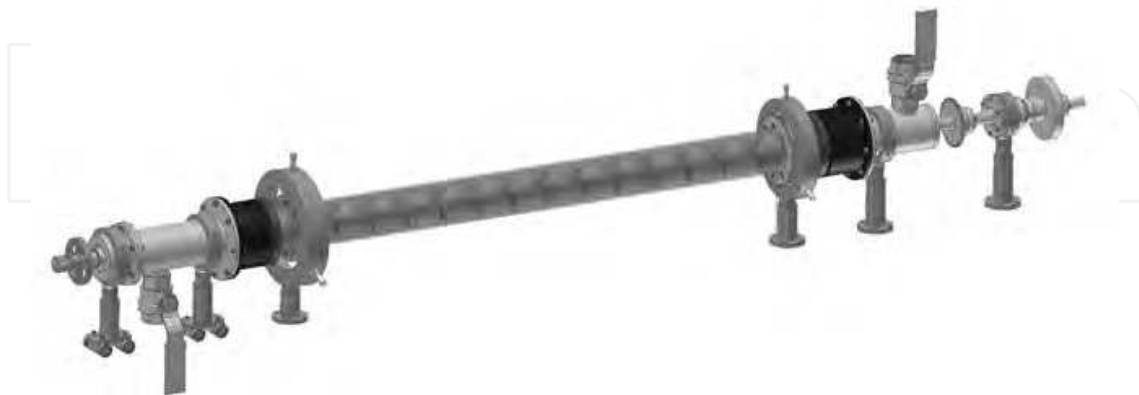
Fig. 24. Sketch of the high temperature rotary kiln reactor for char activation. The operation temperature is 950°C with steam flow and the char throughput amounts to max. 1 kg/h.
