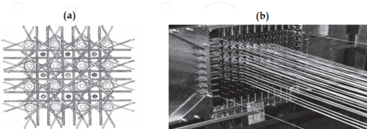
Fig. 18. The fabric (a) and specially designed loom to fabricate the multiaxis 3D fabric (b) (Khokar, 2002b).
