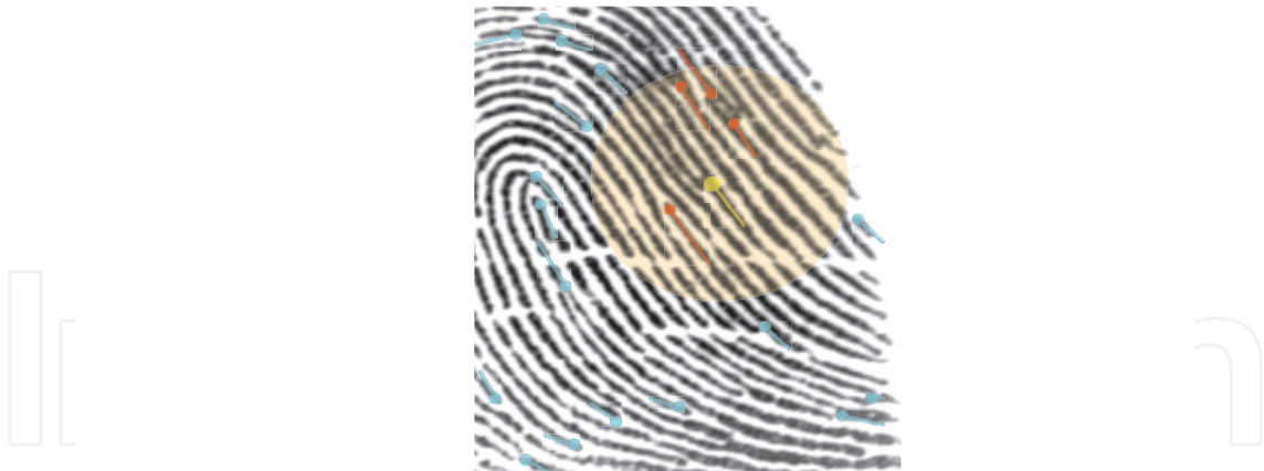
Fig. 12. The \delta -neighbourhood ( \delta = 4 ) for a given minutia (ignoring false crease minutiae).
