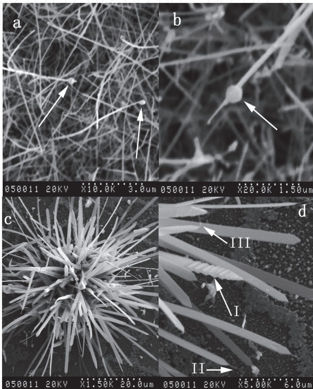
Fig. 17. SEM images of the sample catalyzed by 20 nm MgO thin film as intermediate layer and ammoniated at different temperatures. a, 950 °C; b, 1000 °C; c, 1050°C; d, enlarged picture at the limbic part of c.
