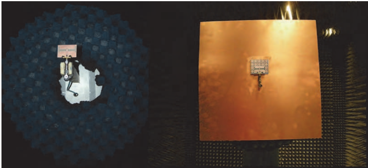
Fig. 8. Measurement set-up in anechoic chamber. Antenna measurement (left) and antenna on AMC over metallic plate measurement (right).
