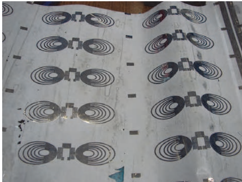
Fig. 7. A hybrid method with gravure printing and vacuum deposition technology
