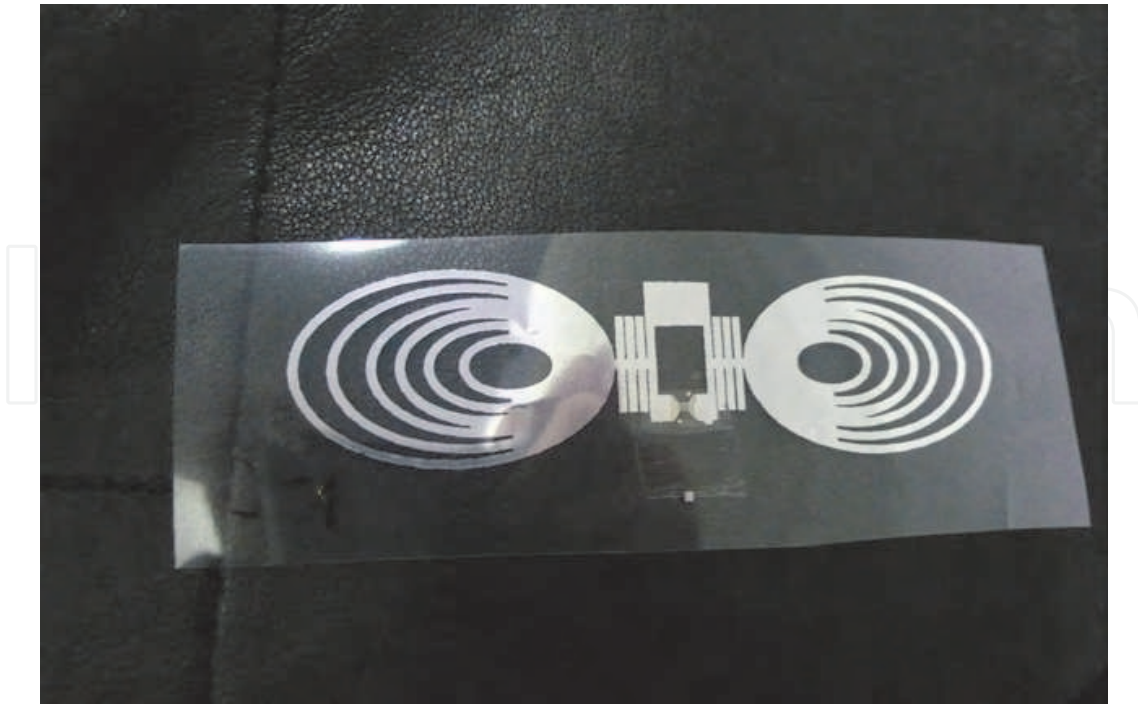
Fig. 14. A tag antenna using a company logo
