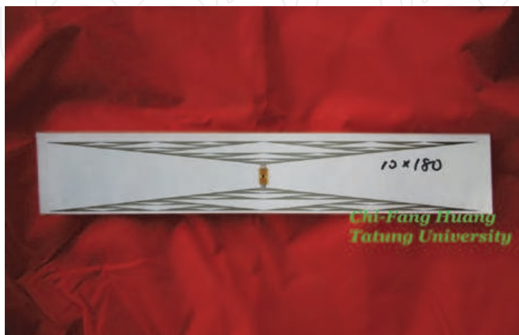
Fig. 5. A single RFID tag of UHF band made by offset printing technology
